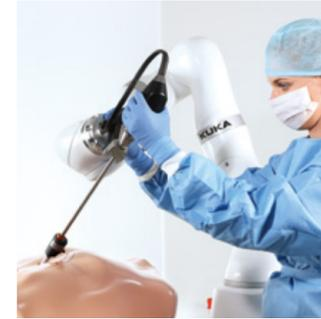
**Minimally invasive surgery:** The highly developed controller enables precise operation with a trocar kinematic system. The user can freely select whether to use the application automatically, interactively or via a telemanipulator.
